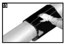
With the green-yellow coloured adhesive side facing down, firmly press the entire closure seal into place. Ensure that the closure is centred evenly over the underlap-overlap sleeve seam. If necessary, add additional heat to the closure underside in cold conditions, using a low flame intensity.
