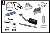
Propane tank, hose, torch & regulator Appropriate tools for surface abrasion Epoxy application accessories & wet film thickness gauge Knife, roller, rags & Canusa approved solvent cleanserDigital thermometer with suitable probe Standard safety equipment: gloves, goggles, hard hat, etc.
