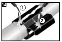
Remove the remaining sleeve release liner and wrap the sleeve loosely around the pipe, ensuring the appropriate
