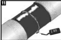
Check the temperature to ensure the preheat has been obtained on the entire pipe circumference. This preheat will substantially cure the epoxy and ensure proper flow and bonding of the sleeve adhesive. Ensure that the epoxy primer is dry to the touch prior to sleeve installation.
