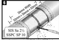
Warm the joint area to 40-50°C (104-120°F) before grit blasting. During high winds or cold ambient conditions (below 15°C (59°F)) pre-warm the joint area to 70°C (158°F) before grit blasting. Thoroughly clean the weld area with a sand or grit blaster to "near white metal" SIS Sa 2½ or equivalent. Abrade the mainline coating adjacent to the weld area to a distance 50mm (2") beyond the sleeve width
