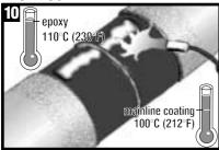
Preheat the epoxy to a temperature of 110°C (230°F) and the abraded mainline coating to be covered by the sleeve to a minimum of 100°C (212°F) with the appropriate propane torch, induction heating or infrared heating equipment. **Do not use an intense flame on the mainline coating.** If a film develops on the mainline coating because of preheat, use a surface abrasion tool to remove it.
