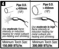
Canusa recommends the use of induction or infrared heating equipment for pipe sizes greater than 760mm (30") 0.D.
